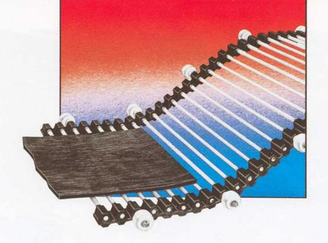
Cooling lines with bar grid conveyors for unvulcanized rubber
